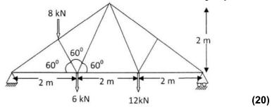
8. Using method of tension Coefficients determine the forces in the members of the space truss shown below. (20)
