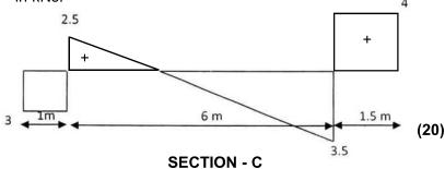
Using double integration method determine the slope at supports and maximum deflection in the beam shown in Figure. The beam has a uniform flexural rigidity EI.
